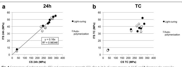
Fig. 4 Comparison of indirect tensile (ITS) and compressive strength (CS) after a 24 h of water storage at 37 °C and b thermocyclic aging for autopolymerized and light-cured specimens
