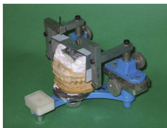
Figure 2 Mandibular position analyzer. The apparatus added to an articulator for the three-dimensional analysis of the mandibular position consists of right and left recording arms with pins into the condylar post holes. The recording frame is attached to the upper cast. The mandibular positions are recorded on the frame by the needles on both sides.
