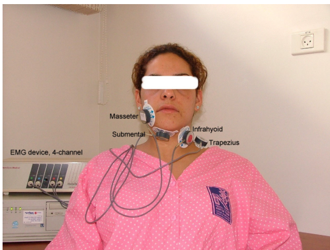
Figure 1 The electroneuromyograph at work. A subject with masseter, submental group, infrahyoid, and trapezius locations of SEMG electrodes.
