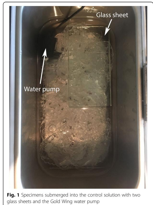
**Fig. 1** Specimens submerged into the control solution with two glass sheets and the Gold Wing water pump
