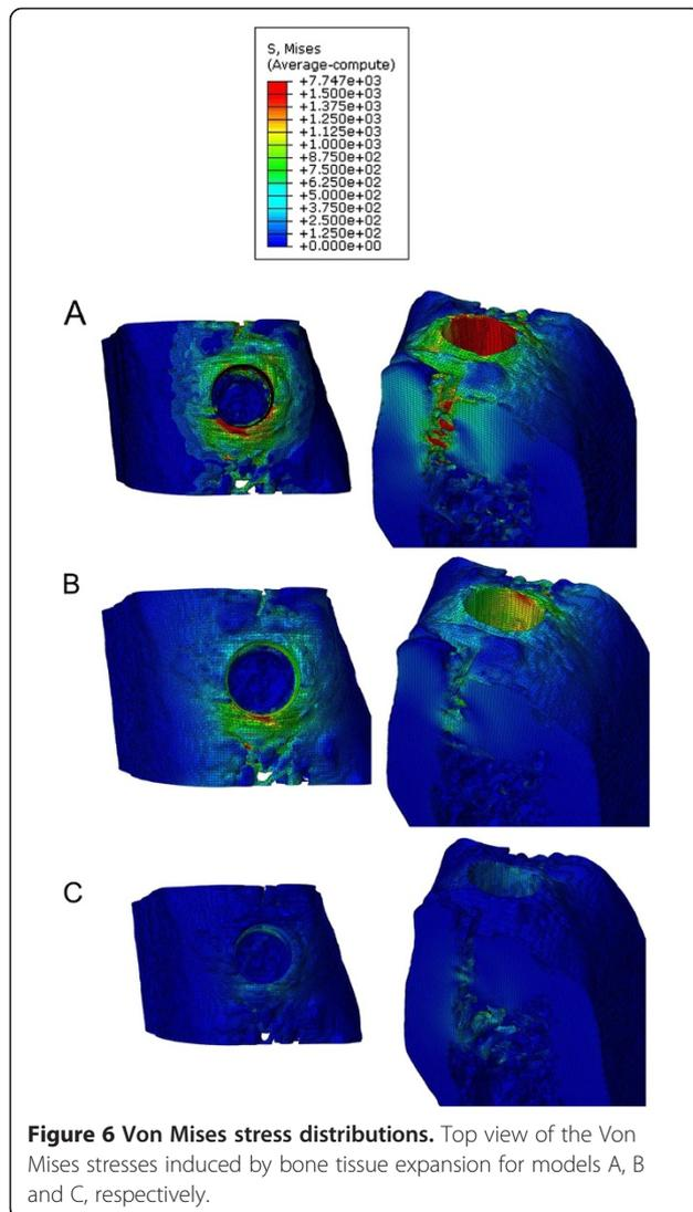
**Figure 6 Von Mises stress distributions.** Top view of the Von Mises stresses induced by bone tissue expansion for models A, B and C, respectively.
